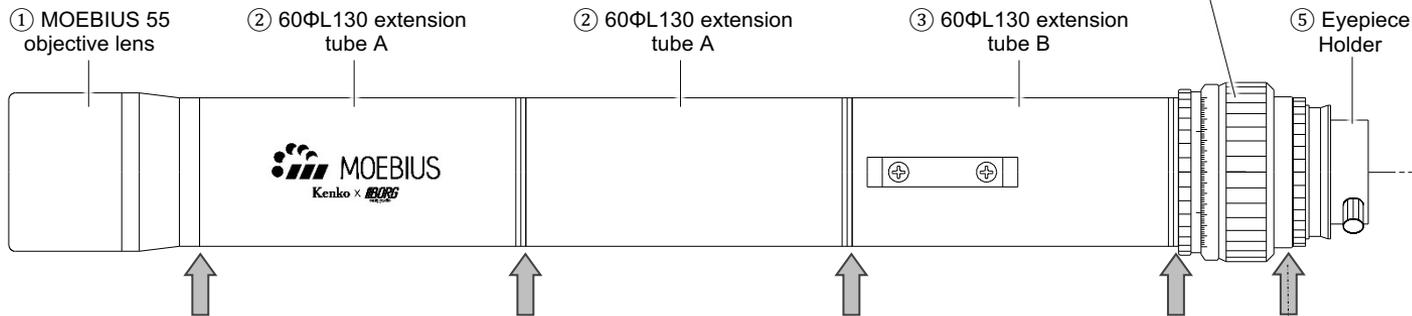
The main unit can be disassembled from the parts indicated with the ↑ symbol in the diagram. When disassembling, please take care not to touch the donut-shaped shielding ring on the inside.
