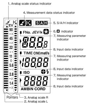
For the purpose of explanation, the diagram above shows all indicators that light up on the LCD.
