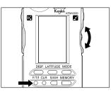
Select two input data parameters among diaphragm shutter speed and ISO by pressing F/T/I button.
