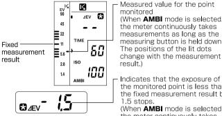
Measured value for the point monitored (When AMBI mode is selected. the meter continuously takes measurements as long as the measuring button is held down. The positions of the lit dots change with the measurement result.)
