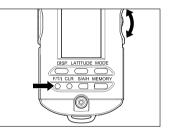
Select two parameters among diaphragm shatter speed and ISO by pressing F/T/I button. Input data by rotating the up/down dial.
