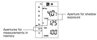
•In the above example, the shadow exposure for the darkest measured area (aperture: F2.0+0.0) was determined.
