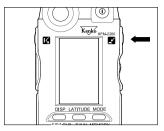
5 Press the incident light measuring button while holding the meter near the subject with the Flat Diffuser facing the main light source.
