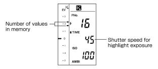
•In the above example, the highlight exposure for the 1/200 sec. of the TIME measurement was determined.
