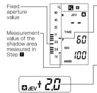
Current measurement value (In AMBI mode, measurements are made continuously while the measuring button is pressed. The positions of the pointers change accordingly.)
