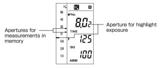
•In the above example, the highlight exposure for the brightest area measured (aperture: F16+0.5 stops) was determined.
