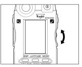
4 Specify the desired shutter speed with the up/down dial.
