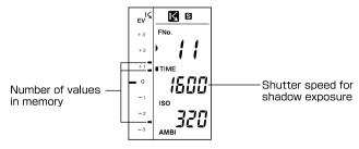
In the above example, the shadow exposure for the 1/250 sec. of TIME measurement was determined.
