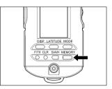
After taking the second measurement, press the MEMORY button to store the second measurement result in memory.
