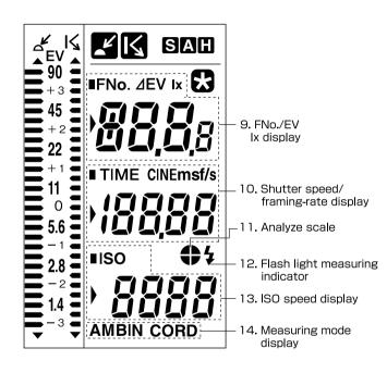
For the purpose of explanation, the diagram above shows all indicators that light up on the LCD.
